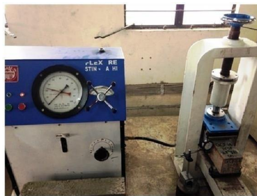
Figure 6 Compression test setup
